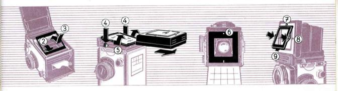
Inserting the Film Mask: Insert the spring loaded side behind the film aperture frame 3, first below 2, then above.
